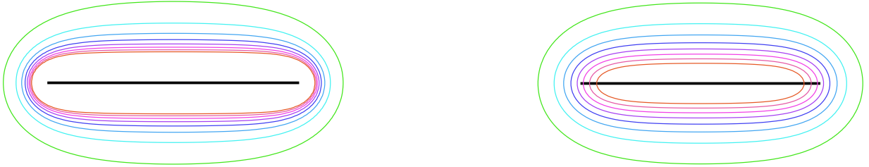
Figure 2: Different level sets of the convolution function for a line segment with a cubic inverse power (left) and the classical Cauchy kernel (right).
