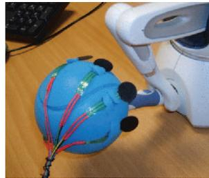
Figure 4: Foam ball with sensors
