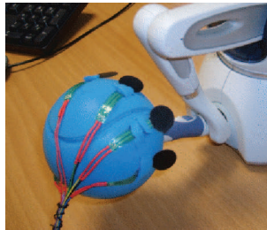
Figure 4: Foam ball with sensors
