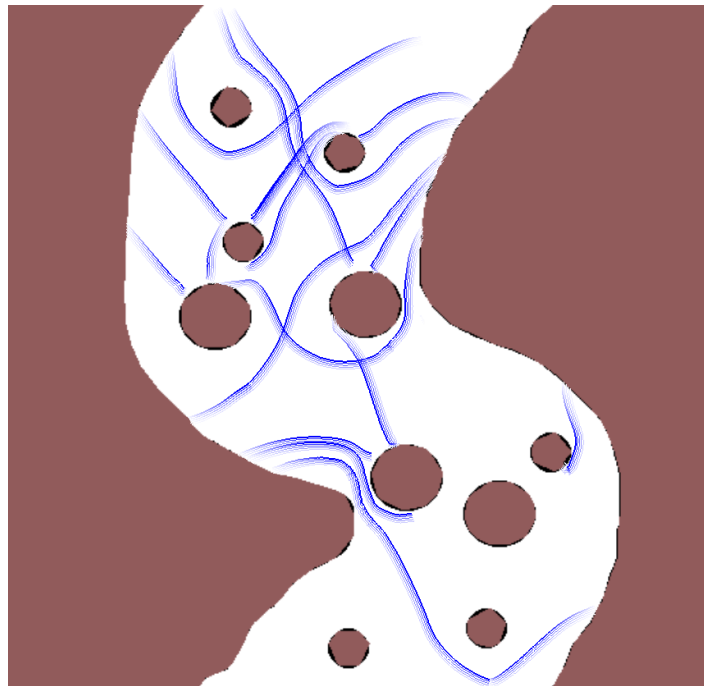
Fig. 11. Shockwaves built upstream and downstream obstacles.
