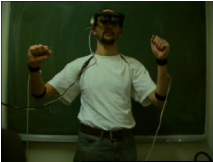
fig7: User with 4 sensors and HMD.
