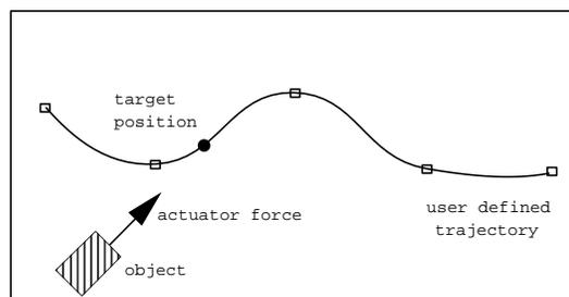
Figure 1: Actuated object guided along a path
