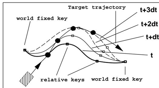
Figure 5: Target motion for a relative path
