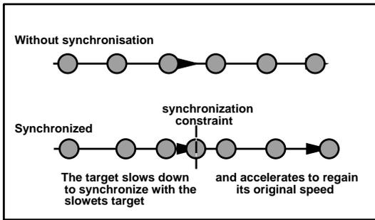
Figure 8: Target Speed Variations due to synchronization
