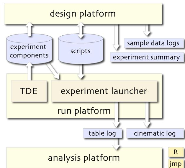
**Figure 1. Touchstone architecture: design, run and analysis platforms**
