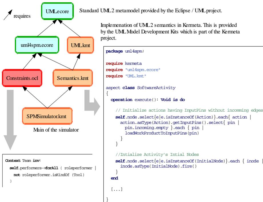
Fig. 7. Weaving Executability to The UML4SPM Metamodel
