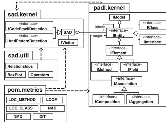
Fig. 8. Architecture of the SMELFW framework.
