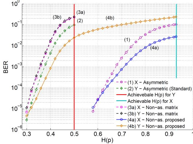
Fig. 3. Performance of the non-asymmetric SW codec, for a non-uniform source  $X \sim \mathcal{B}(p_X = 0.12)$ .  $H(X|Y) = 0.5$  occurs for  $H(p) = 0.93$ , whereas  $H(Y|X) = 0.5$  occurs for  $H(p) = 0.5$ . This difference comes from the BSC between the sources which is not symmetric in the two sources.
