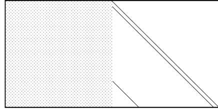
Fig. 2. Shape of the designed LDPC code's parity-check matrix, inspired by the structure of IRA codes. The columns forming the weight-two and weight-three columns are chosen as the triangular part  $\mathbf{B}$ .
