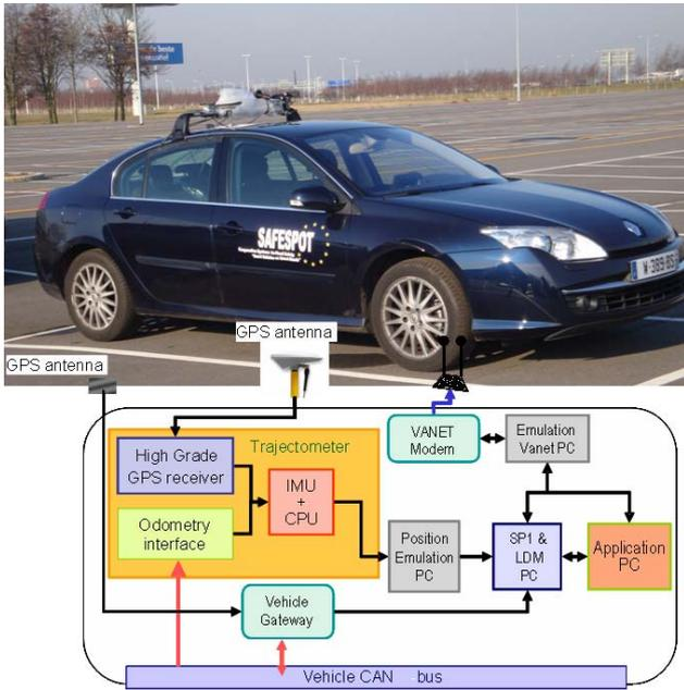
Figure 6 : Schematic representation of the implemented system
