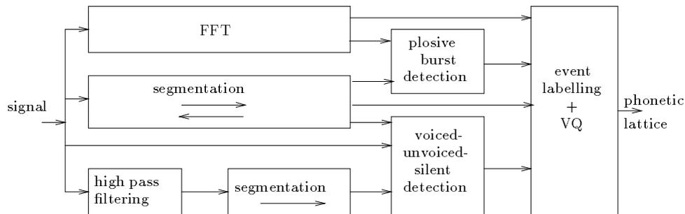
Figure 10: *Modular description of an acoustic-phonetic decoder*
