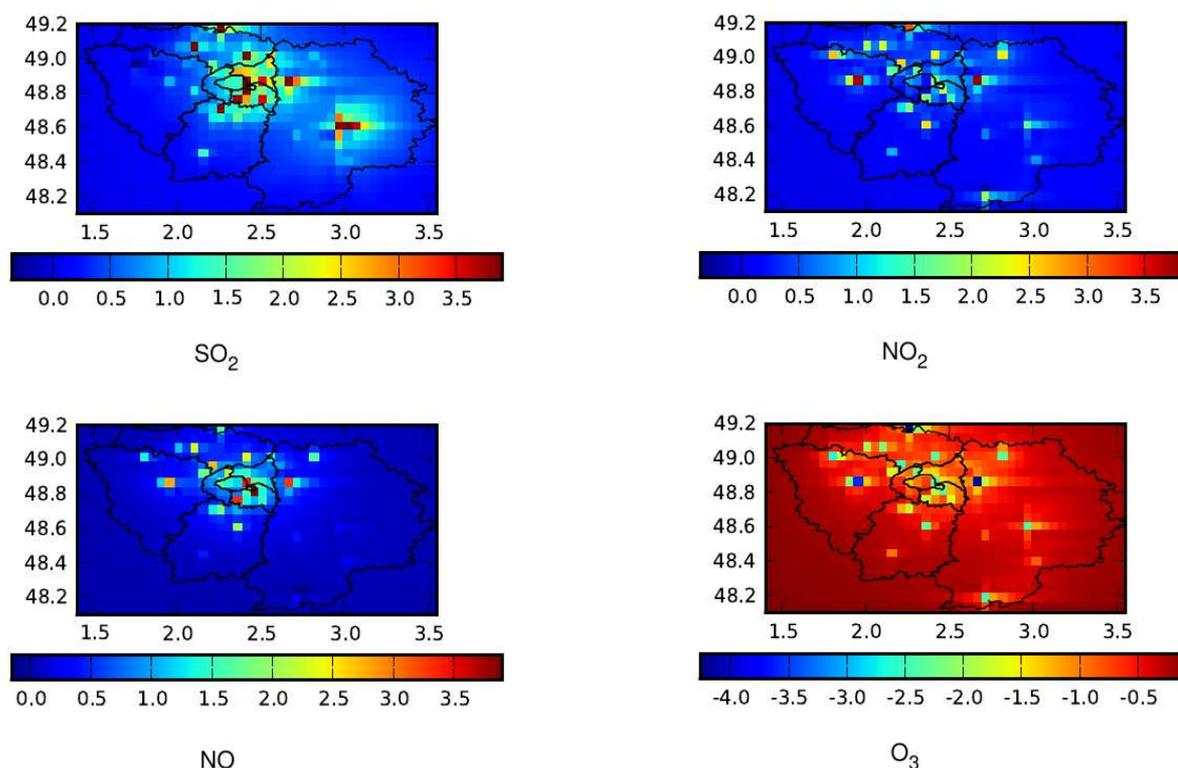
Figure 2. Differences between mean ground concentrations with Polair3D alone, and with plume-in-grid treatment. Mean values over six months, in micrograms per cubic meter.
