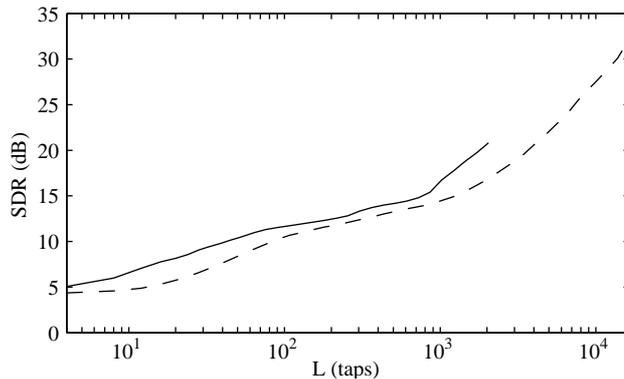
Figure 4. Average performance of various source image demixing filters on determined two-source mixtures with reverberation time  $RT = 250$  ms. Plain: time-domain oracle demixing filters of length  $L$ . Dashed: near-optimal frequency-domain demixing filters with  $L$  frequency bins. Long oracle filters could not be estimated due to large memory requirements.
