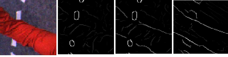
Fig. 3. (a) The arm is visible from the top view. (b) Standard Canny filter reveals markings on the ground and foldings of the clothings. (c) Color Canny filter partially detects the arm contours. (d) Anisotropic Gaussian color filter reveals the full arm contours.
