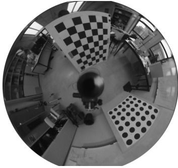
Fig. 3. Monocular image of a calibration chessboard.
