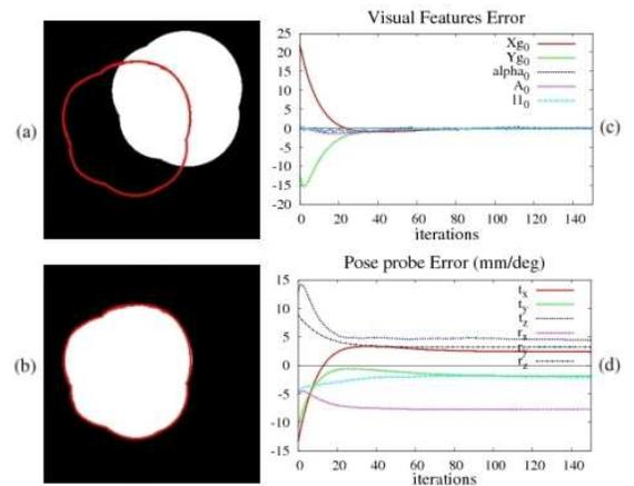
Fig. 2. (a), (b) Initial and final images of the probe. (c) Exponential decrease of the visual features errors. (d) Probe pose error in mm and deg. (the  $\theta \mathbf{u}$  representation is used to describe the orientation).
