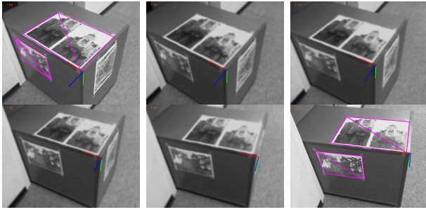
Fig. 4. Occlusion simulation example. First and last image show images before and after occlusion. This occlusion lasts more than 3 seconds. Thanks to the inertial sensors, intermediate images shows that the pose is efficiently estimated.
