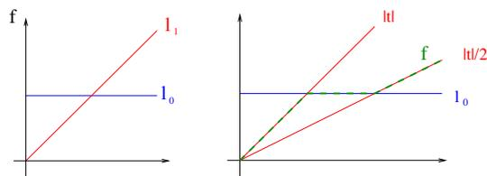
**Fig. 1.** (a) The “nice” functions  $f_0(t)$  and  $f_1(t)$  corresponding to the  $\ell^0$  and the  $\ell^1$  norm (b) An “exotic” sparsity measure, based on a mix of the  $\ell^0$  and  $\ell^1$  measures plotted in (a).
