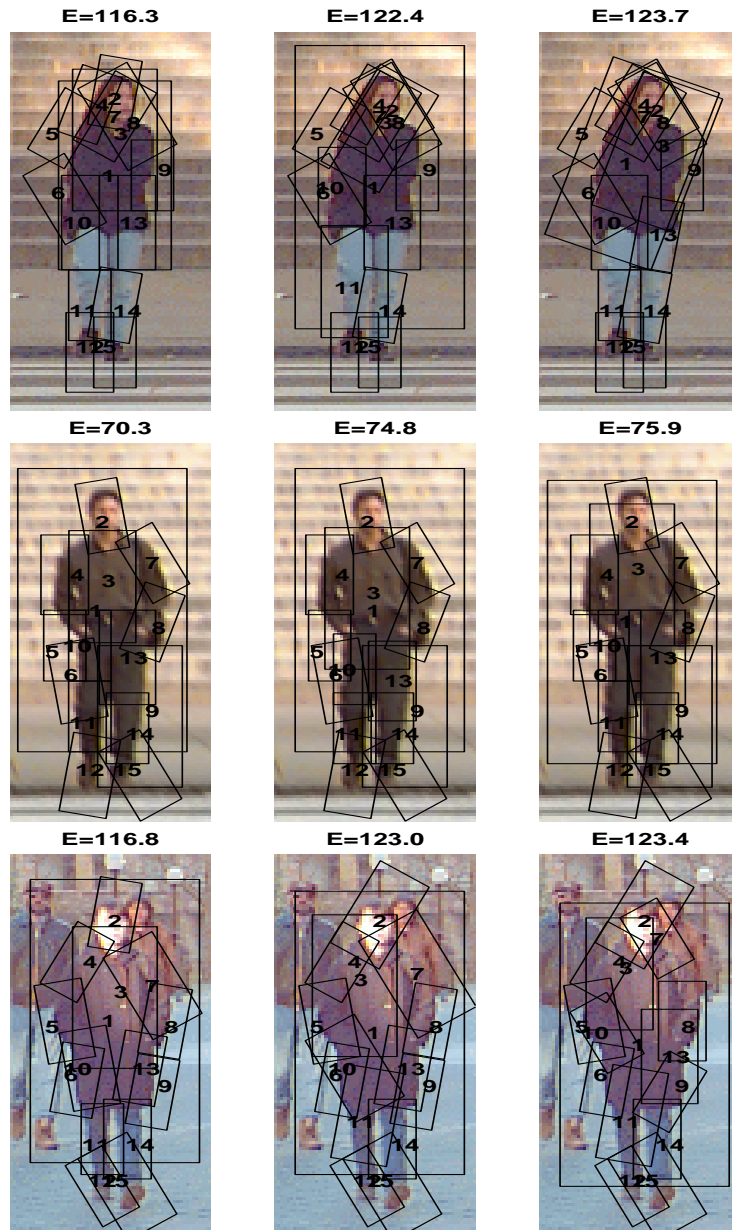
Figure 6. Ranked detections and their energies, using the learned body model and SVM scores.
