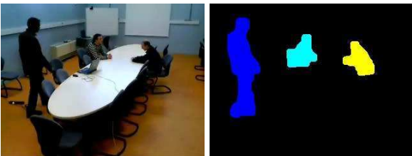
Fig. 1 Example of result obtained after background subtraction and post-processing (one color per object).
