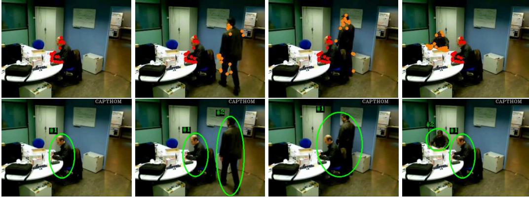
Fig. 3 Illustration of tracking result with a partial occlusion. The first row corresponds to input images with interest points associated with each object (one color per object) and the second row corresponds to the tracking result with a label consistent in time for each object.
