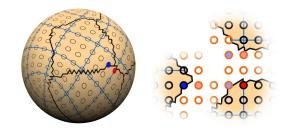
**Figure 1:** Neighboring texels on the surface (left, red/blue dots) are not neighbors in the atlas (right). To make the seam invisible, texels have to align across chart boundaries and their colors have to be duplicated (light colored texels).
