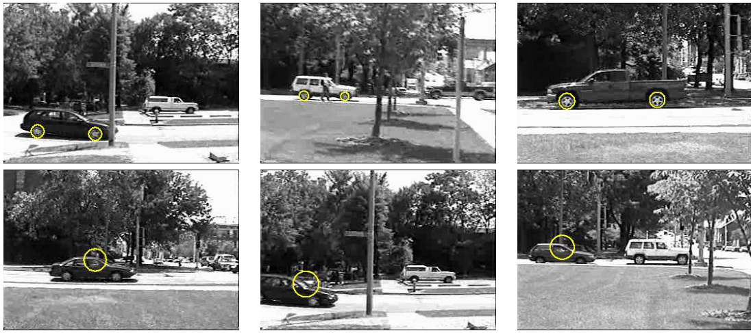
Figure 2. A few images of two different clusters. The first row shows a cluster which represents “tires”. The second row shows a cluster which contains regions detected in the “front window”.
