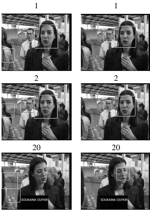
Figure 3. The first column : frame-by-frame detector. The second column : “temporal” detector. The frame numbers are marked above the images.
