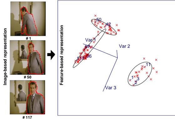
Figure 1: *Illustration of the content variation of a non-rigid tracked object and its modeling in the three principal components of the RGB histogram space by a mixture of three Gaussians. Three key-frames among 117 occurrences of the object are depicted and the covariance ellipses are also displayed.*
