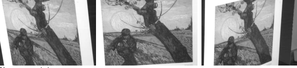
Figure 11: Viewpoint change sequence: from left to right image 0, 7 (reference image) and 15. Image 0 is taken at the rightmost position of the camera. For image 7 the camera is in front of the painting. Image 15 is taken at the leftmost position.
