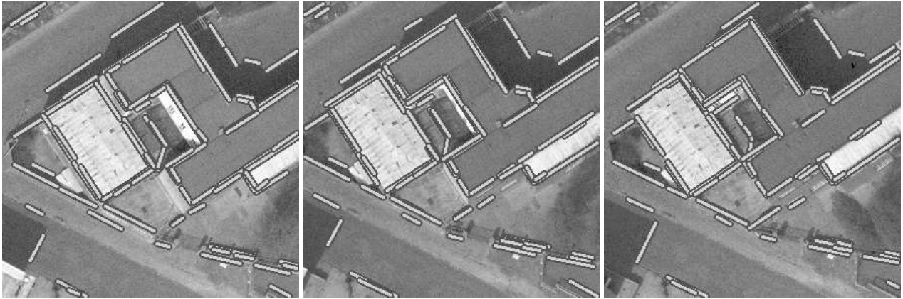
Figure 7. Matching across three views using both line transfer and a short range matching correlation score. All of the 89 matches obtained are correct.
