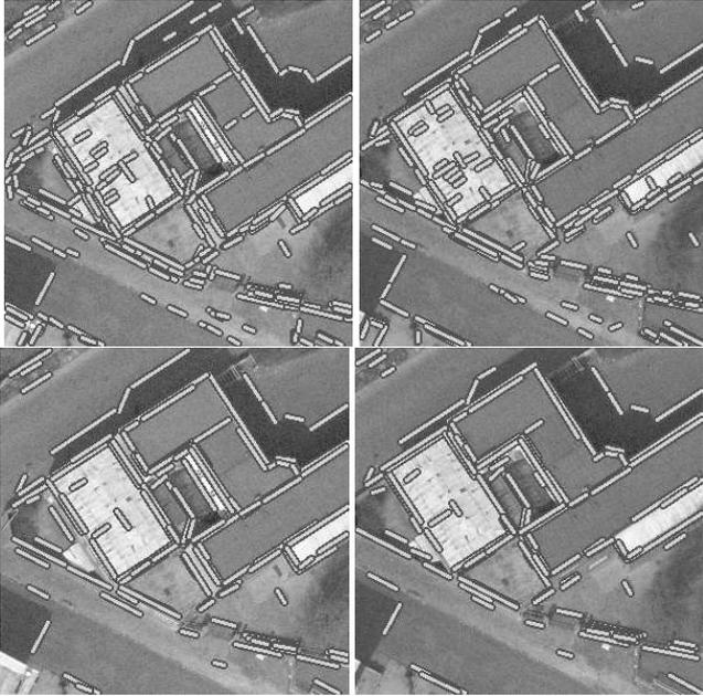
**Figure 1.** Upper pair: extracted lines segments superimposed on the left/right images; Lower pair: matched segments using the short range motion algorithm. 97.5% of the 122 matches shown are correct.
