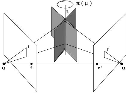
**Figure 3.** Image lines  $l$  and  $l'$  determine a line  $L$  in 3-space. The line  $L$  is contained in a one parameter family of planes  $\pi(\mu)$ . This family of planes induces a one parameter family of homographies between the images.
