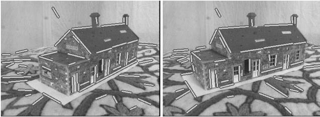
**Figure 6.** Matched line segments using the long range motion algorithm. There is significantly different foreshortening between the planes of the house in the two images. 77% of the 53 lines shown are correctly matched.
