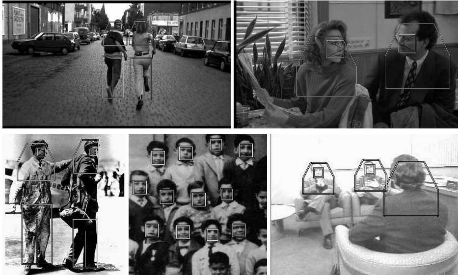
Fig. 7. Human detection with the joint model. Top row: images from movies “Run Lola Run” and “Groundhog Day”. Bottom row: images from MIT-CMU database.
