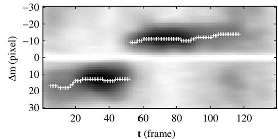
Fig. 4.  $\dot{X}^\times$ , the result of the correlation of the positive and negative derivative part ( $\dot{X}'^+$  and  $\dot{X}'^-$ ) with respect to the  $x$ -axis; the sign “+” marks a local maximum above the determined threshold.
