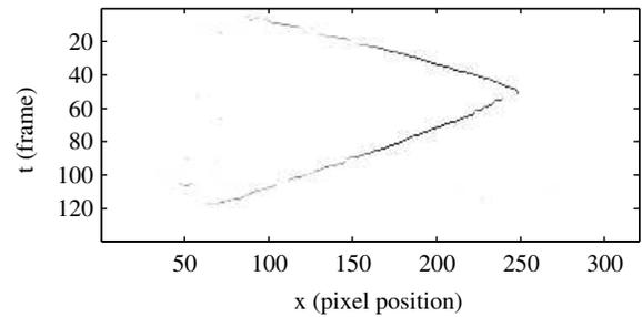
(d)  $\dot{X}''$ , the resulting signal after shifting and multiplying it by itself as well as the application of morphological operators; the motion trajectory has been thinned out, only some noise particles remain.
