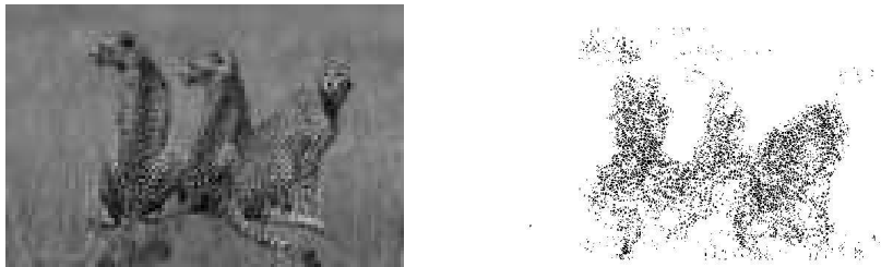
Figure 6: Localization of the cheetah model for one of the test images (left). Locations with high probability scores are displayed in black (right).
