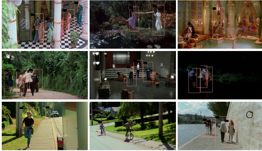
Fig. 7. Sample detections on Test Set 2 from the combined SHOG + IMHcd detector trained on Set 1 + Static . Note the variations in pose, appearance, background and lightning.
