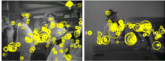
Figure 5. Space-time interest points detected for two video frames with human actions hand shake (left) and get out car (right).
