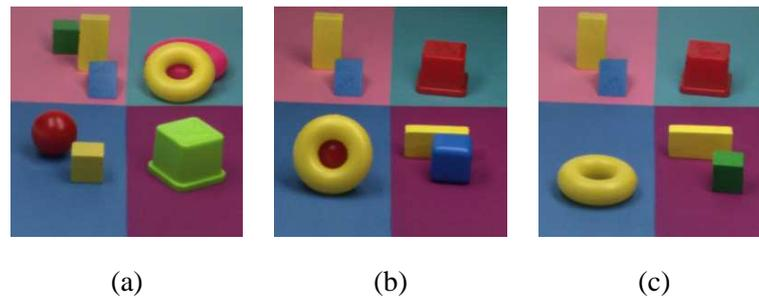
Figure 1.9: (a) Example image 1, (b) Example image 2, (c) Example image 3. The images are recorded in 3 *RGB*-colors with the aid of the SONY XC-003P CCD color camera (3 chips) and the Matrox Magic Color frame grabber. Two light sources of average day-light color are used to illuminate the objects in the scene.
