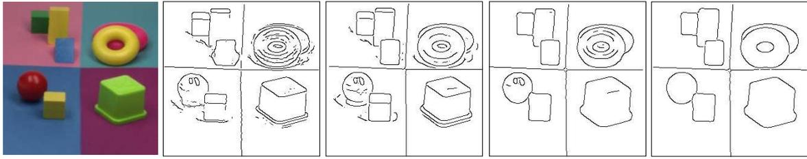
Figure 1.1: (a) Input image with Canny edge detection based on successively, (b) luminance derivative, (c) *RGB* derivatives, (d) the shadow-shading quasi-invariant, (e) the shadow-shading-specular quasi-invariant.
