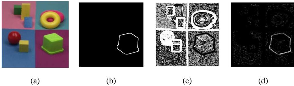
Figure 1.3: (a) Lab image, (b) groundtruth for learning edges. Input image for the edge and corner detection, on the left the edge is indicated for the learning algorithm. (c) The  $\chi$ -squared error of the transformed image and the predicted expected value, here the edges have a very low intensity, (d) the local signal-to-noise ratio for the transformed image. The edges have a higher ratio.
