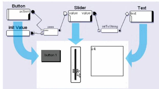
Figure 14: Connection of manipulators devices. The button resets the slider and the slider value is displayed in the text zone.
