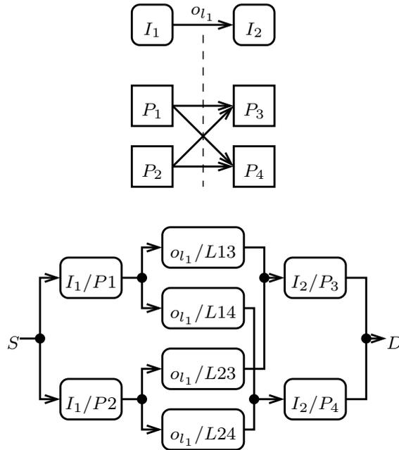
Figure 4: A mapping of two intervals ( $I_1$  and  $I_2$ ) on four processors ( $P_1$  to  $P_4$ ) and its RBD which has no particular form.
