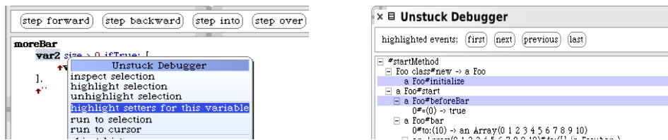
Figure 3: Left: highlight the modifiers of a variable over the context menu in the source view. Right: the result of the action made on the left side: highlighted methods in which var2 was modified ( i.e. , changed the value)
