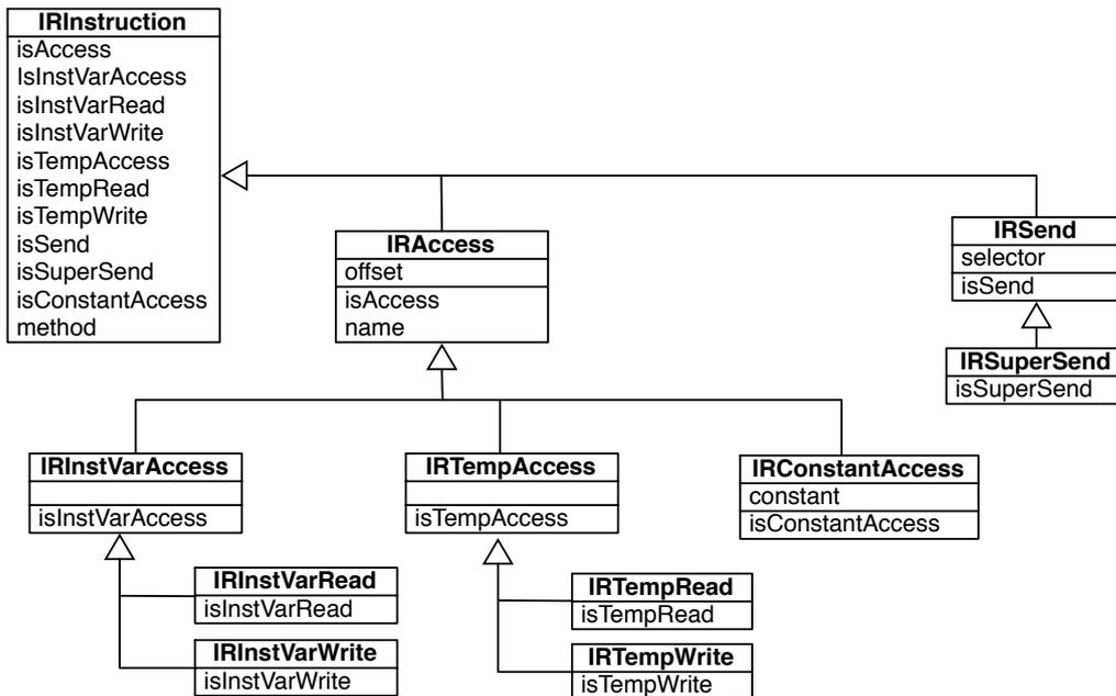
Fig. 1. Structural model of instructions in BYTESURGEON.
