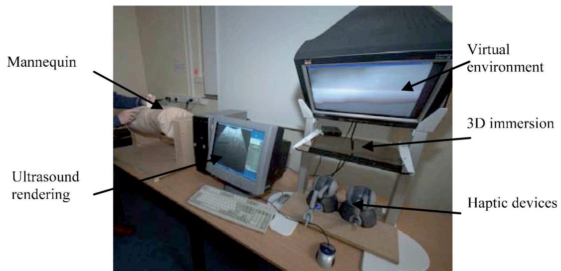
Figure 1. Ultrasound-guided liver biopsy simulator components.
