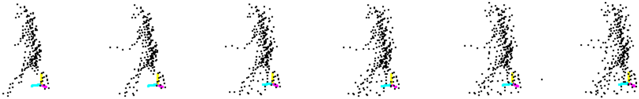
Fig. 5. Dynamic mapping: result of iterative motion estimation and accumulation of measurements when passing by a pedestrian (with attached local coordinate frame). Non-rigid objects will be mapped with more noise but data association still benefits from dynamic mapping
