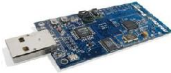
Figure 5: Tmote SKY platform from Crossbow
