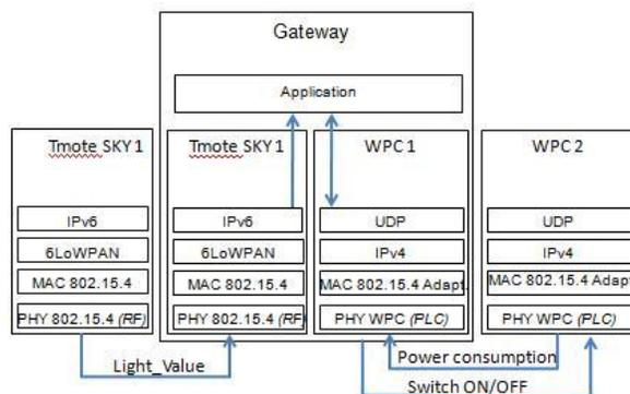
Figure 9: Communication layers
