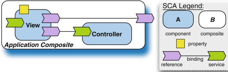
Fig. 9.2 Overview of the SCA component model
