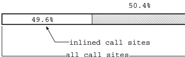
As seen previously, inlining may occur for a monomorphic site as well as inside a multi-branch dispatch function. For a total of 14,376 inlined sites, 1,603 are inside dispatch functions:
