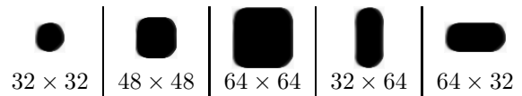
Fig. 9. The diffusion-based controller resulting from an optimization for the 32 \times 32 disc target is used in different grid sizes. The development still features a stable attractor for all grid geometries. Note the non-homothetic scaling of the pattern: the corners keep their round shape, while the side limits between black and white remain straight.
