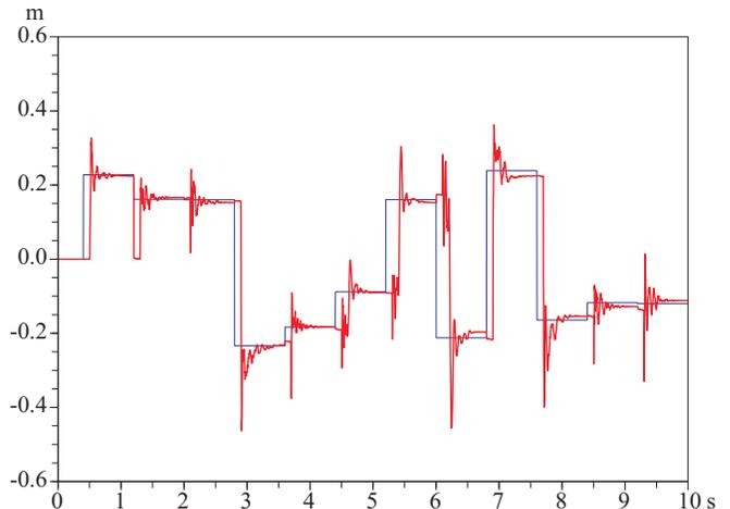
Fig. 7. Length of the current step,  $\delta_{jk}$ , realized by the demonstrator (in thin blue line), chosen randomly, and imitation realized synchronously by the imitator (thick red line). The robots are using different controller and only sensors on ankles are used.
