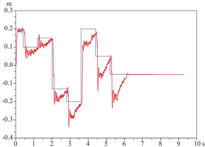
Fig. 3. Length of the next step,  $\delta_{j_{k+1}}$ , planned by the demonstrator (thin blue line), chosen randomly, and guess made by the imitator (thick red line). The robots are using the same controller.
