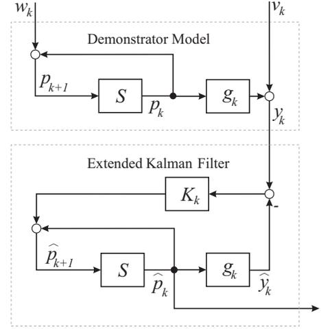
Fig. 1. A simple stochastic process representing the evolution of the control parameters  $p$  (the block  $S$  is a simple time shift), and the Extended Kalman Filter which is used to identify the value of this parameter with the help of sensor signals  $y$ .
