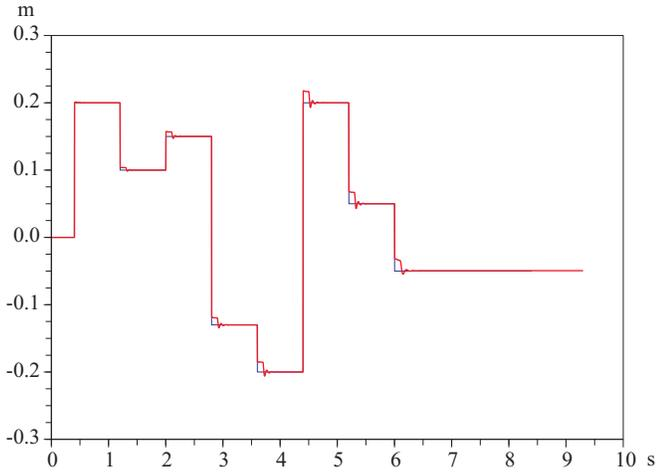
Fig. 2. Length of the current step,  $\delta_{j_k}$ , realized by the demonstrator (in thin blue line), chosen randomly, and imitation realized synchronously by the imitator (thick red line). The robots are using the same controller.
