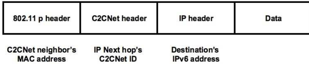
Fig. 2. GeoNet packet encapsulation
