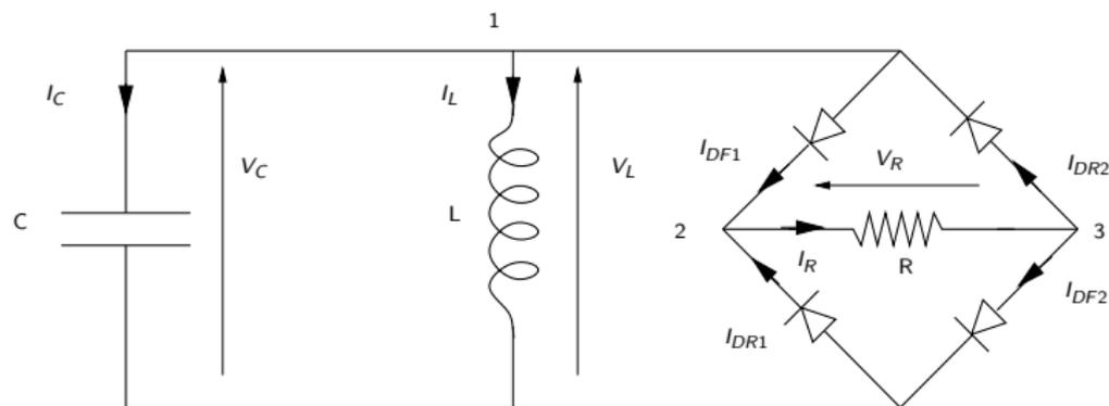
Figure: The Diode-bridge rectifier
