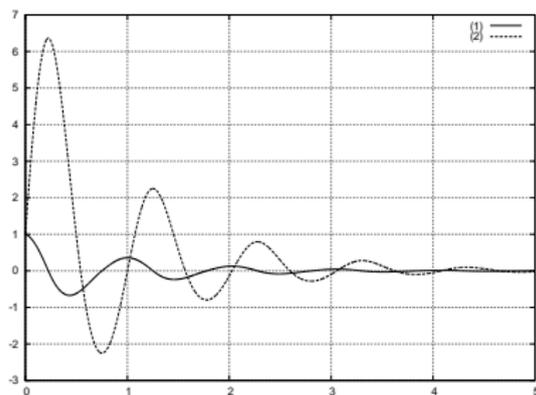
(a) state versus time  $v_L$  and  $i_L$
