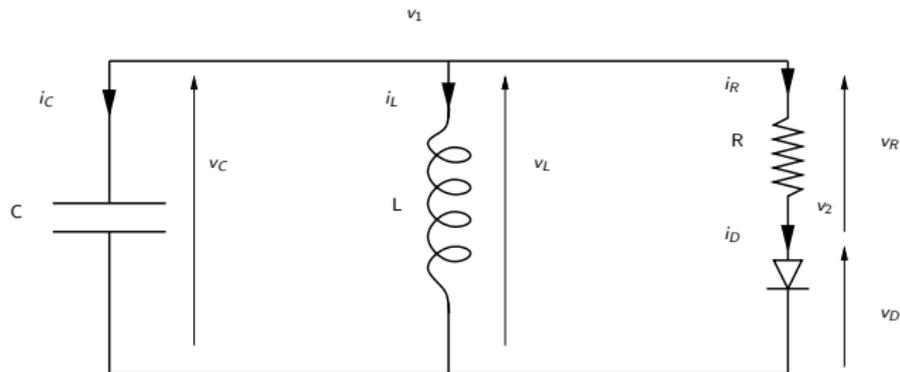
Figure: Electrical oscillator with half-wave rectifier
