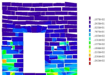
Figure: VON MISES stresses
