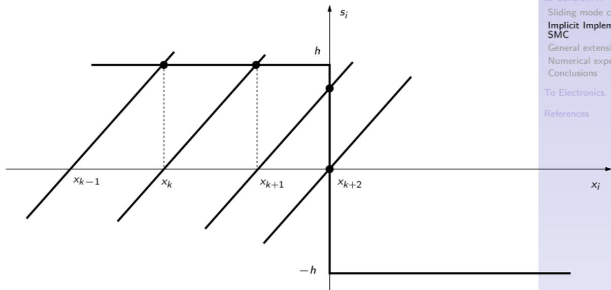
Figure: Iterations of the backward Euler method.
