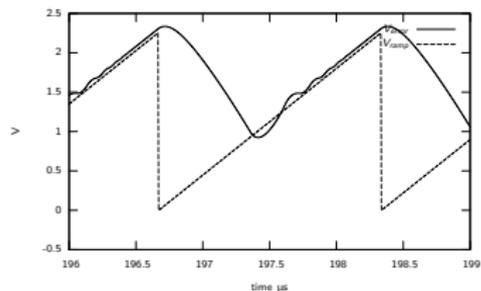
(b)  $V_{\text{ramp}}$  and  $V_{\text{error}}$
