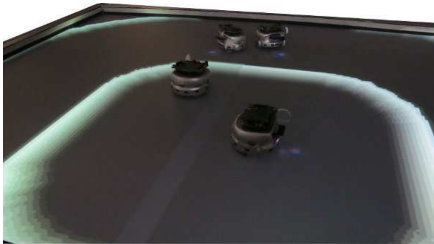
Fig. 7. Snapshot of an experiment using the Khepera robots on the interactive ROMEA table. The experiment uses a circular neighborhood with radius 2.5 and M=6
