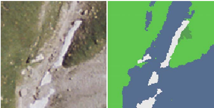
Fig. 40.6 Image classification correction Original aerial image ( left ), class map ( right )
