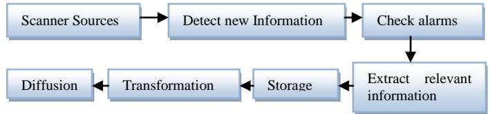
**Figure 5:** Alarm Process
