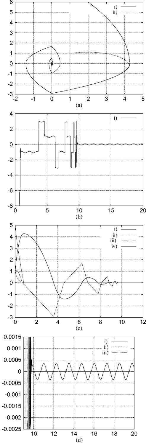
Fig. 6. Simulation of (60) with  $\varphi(t) = \phi \sin(\omega t)$ ,  $\phi = 0.1$ ,  $\omega = 5$ . (a) Phase portrait. i) State  $x_k$  versus  $y_k$  ii) observer  $\hat{x}_k$  versus  $\hat{y}_k$ ; (b) control versus time i)  $u_k$ ; (c) state and error versus time i)  $\hat{x}_k$  ii)  $\hat{y}_k$  iii)  $e_{1,k}$  iv)  $e_{2,k}$ . (d) Sliding variable versus time. i)  $\text{sgn}(\hat{y}_k)$  ii)  $\text{sgn}(e_{1,k})$  iii)  $\text{sgn}(\hat{x}_k)$ .
