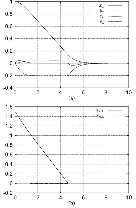
Fig. 4. Simulation of (44) with  $\varphi(t) = 0$ . (a) State versus time. (b) Sliding variable  $s(t)$ .
