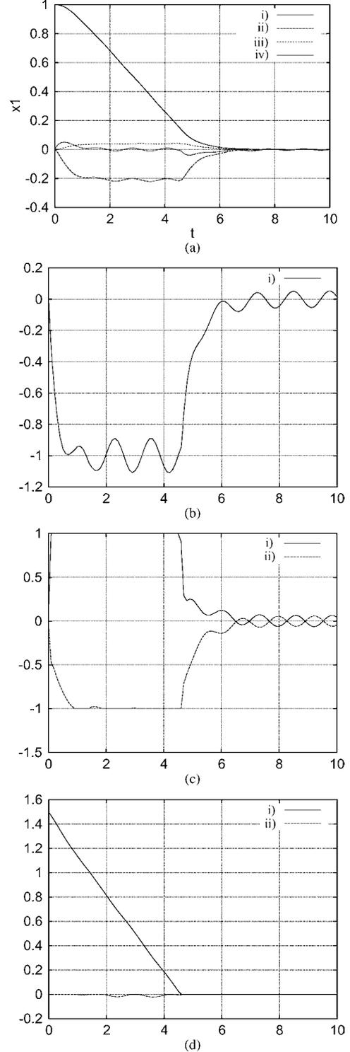
Fig. 5. Simulation of (44) with  $\varphi(t) = \phi \sin(\omega t)$ ,  $\phi = 0.1$ ,  $\omega = 5$ . (a) State versus time (fine sampling): i)  $x_k$ , ii)  $\hat{x}_k$ , iii)  $e_k$ , iv)  $\hat{e}_k$ . (b) Control versus time i)  $u_k$ . (c) Multiplier versus time: i)  $\tau_{1,k}$ , ii)  $\tau_{2,k}$ . (d) Sliding variable i)  $s_{x,k}$  ii)  $s_{e,k}$ .
