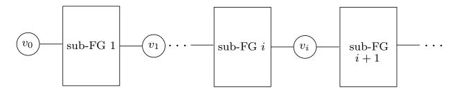
Figure 1. FG well-suited to a sequential implementation of the ML criterion.
